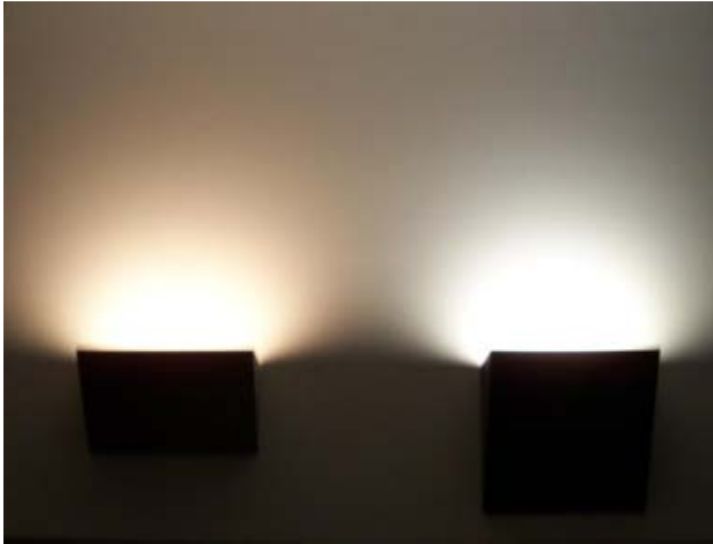
Figure 24: Comparison of halogen (left) to XP-G prototype sconce (right)
